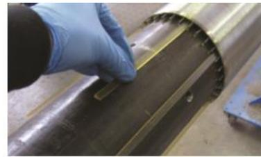
**Fig. 1 - RESMAN tracers are easily integrated into the screens, eliminating design complexity and operational risk**
