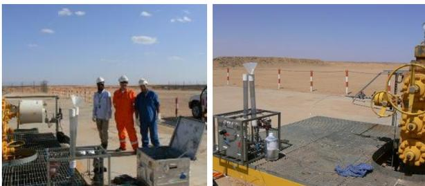
**Fig. 1 – On site In Salah: RESMAN's injected CCS tracers to monitor CO<sub>2</sub> movement from CCS injectors.**
