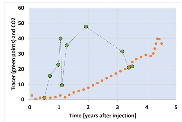
**Fig. 2 – Tracer data (points) and CO<sub>2</sub> as function of time in observation wells in the K12-B project, where RESMAN's CO<sub>2</sub> tracers were first piloted. (Data reproduced from Vanderweijer et al., 2011 - Energy Procedia 4:5471-5478).**
