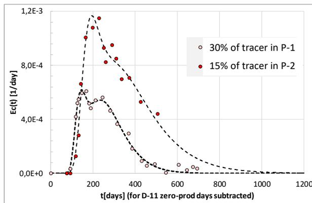
**Fig. 1 - Tracer from one injector in two of the adjacent producers in the field. The symbols correspond to measured tracer data, transformed into a residence time distribution (RTD). The dashed lines correspond to RESMAN's model curves, used to extrapolate the RTD beyond the last data points.**
