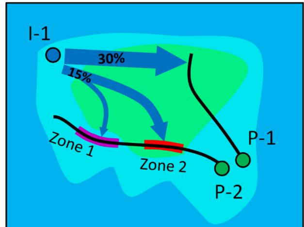
**Fig. 2 - Summary of flow characteristics from one injector (I-1) towards two producers (P-1 and P-2) in the field. Flow directions and magnitude are illustrated as arrows where the arrow widths are proportional to the percentage of water from the injector towards each producer.**
