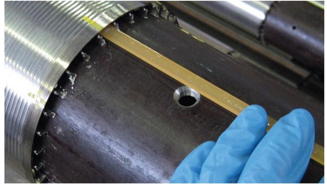
Fig. 3 - When contacted by the target fluid, RESMAN Intelligent Tracers (red strips) release their chemical signature (red dots) independent of flow and at lab-designed rates.
